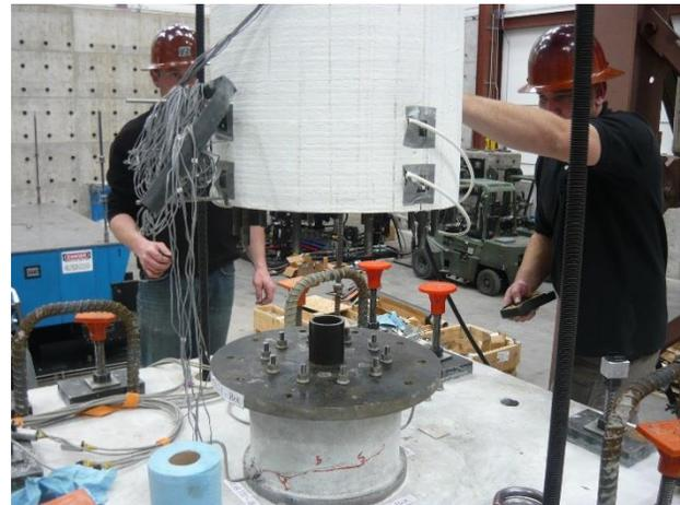
*Three 1/4-scale column models were tested under simulated earthquake motions at the multi-shake-table facility at the University of Nevada, Reno. The test variables included the type of replaceable element at the base of the column and the type of reinforcing superelastic alloy, and each column was tested, disassembled, reassembled, and tested again.*
