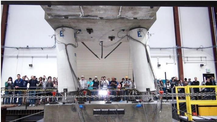
*The new system was successfully evaluated by testing a two-span bridge model and the bridge was then disassembled and reassembled, and subsequently retested*
